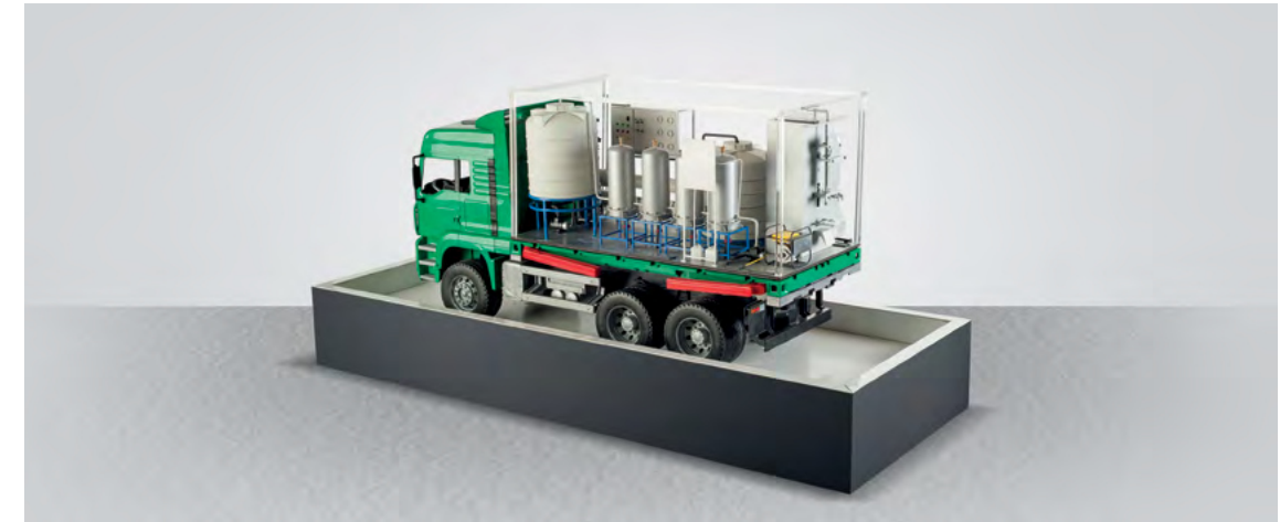
A Portable Turbidity Removing System
